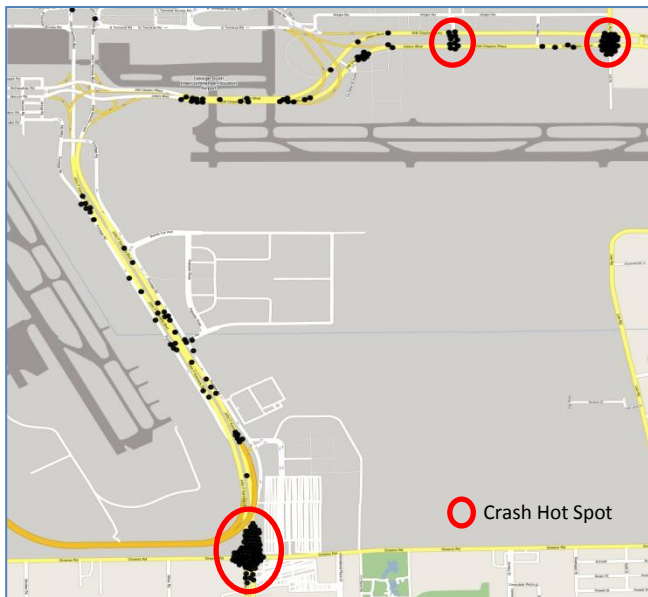
Fig 5.1 - A crash map can help identify high-accident locations and suggest causes and mitigation options.
