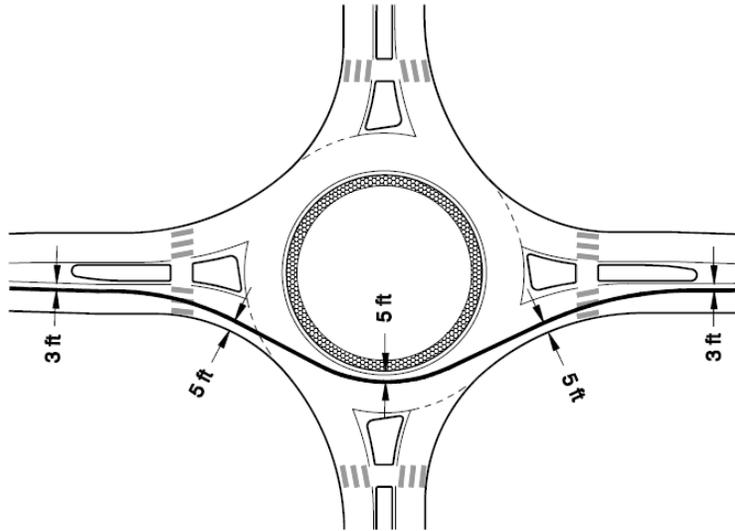
Figure 7.10.3 – Measurement of Fastest Path
