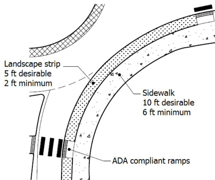
Figure 7.10.8 – Sidewalk Dimensions
