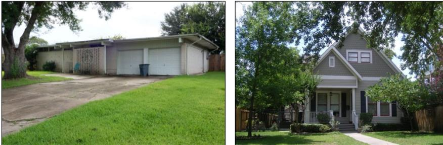
Figure 7. Extreme roof pitches: (left) a nearly flat 1/12 roof in League City, Texas; (right) a very steep 10/12 roof in Houston Heights, Houston, Texas (McDoux)
